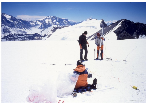
Figure 2.3: Shallow core drilling on Glaciar Esmeralda, Cerro Plomo.
