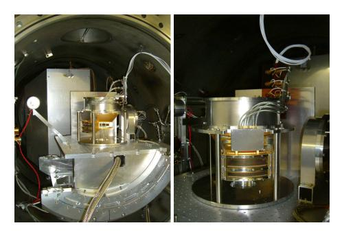
Figure 3.4: Mounting of PLASTIC ESEA in CASYMS facility. The instrument was mounted upside down, the TOF-section would be above. The ion beam comes from the left hand side. On the right picture the theta table can be seen which allows turning around the  $\theta_{CASYMS}$ -axis in figure 3.2
