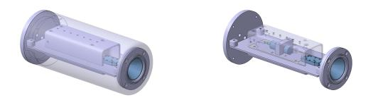
Figure 4.7: Drawing of LaserCEM II. Well visible the faraday cage protecting the laser diode and proximity electronics from discharges. Drawings courtesy of K. Bratschi, UBe.
