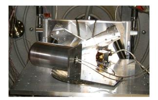
Figure 4.10: The LaserCEM II mounted in MEFISTO instrument chamber for partial discharge tests. The LaserCEM is placed inside an aluminium box. The distance test box to the LaserCEM is at least 2 cm.
