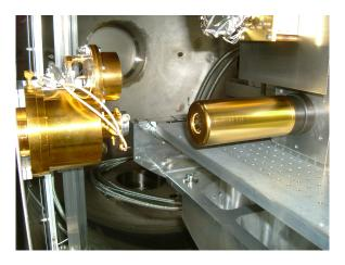
Figure 4.11: The LaserCEM II mounted in CASYMS instrument chamber. The aperture points towards ion beam. On the left side the beam scanner can be seen. A plate with a 3.61 mm diameter pinhole is mounted on the beam scanner allowing position mapping. See text for explanations.
