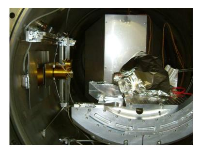
Figure C.1: Experimental setup for MCP detector efficiency measurements in CASYMS. The MCP detector was mounted in the middle of the chamber. The ion beam can be blocked by the CASYMS beam scanner. To prevent ions passing the beam scanner a plate with a pinhole with diameter 3.6 mm was mounted on the movable beam scanner.
