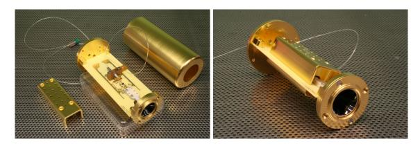
Figure 4.8: Pictures of LaserCEM II Left: Faraday cage of laser diode and electronics removed. Right: Assembled LaserCEM II without cover and grids in front of the CEM aperture. Courtesy Jürg Jost, UBe.
