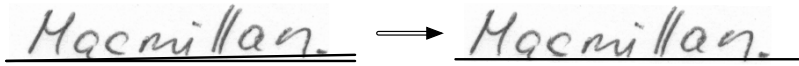
Figure 3.1 Example illustrating the skew correction. The image on the left side is the original input image. The imaginary line on which the handwriting is written is estimated. A rotation corrects the line to become horizontal. The result is shown in the right image.
