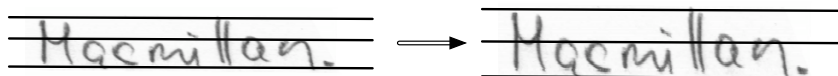
Figure 3.3 Example illustrating the normalisation of the writing regions. The parts of the text line image, i.e. descender, middle, and ascender part are estimated. In this example no descender part is present. The parts are then scaled to predefined height.
