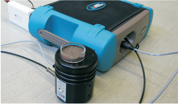
Figure 2.3 Used laboratory measuring setup: FieldSpec 3 spectrometer, muglight, and petri dish containing soil material placed atop of the muglight for the spectral measurement.
