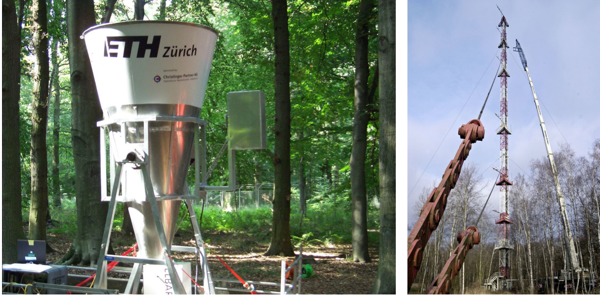
Fig. 3. ELBARA looking at the forest canopy from below (left), and the installation of ELBARA on the 100-m-high platform of the meteorological tower (right).
