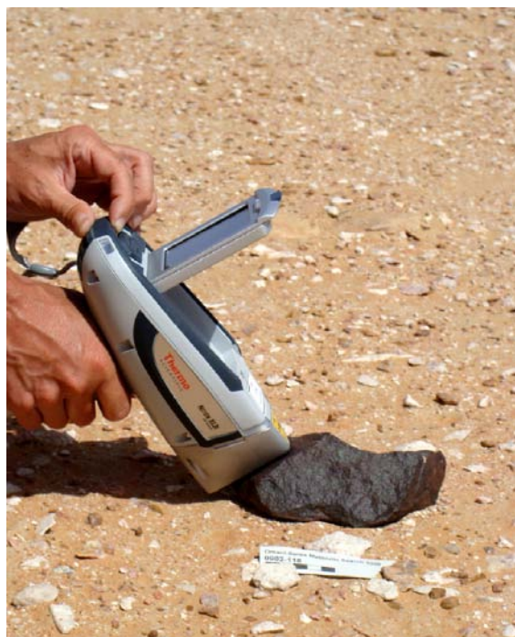
Figure 3.2. In situ HHXRF analysis of a meteorite (RaS 309) discovered in the desert of Oman. Note the high contrast between the dark meteorite and the light colored soil.
