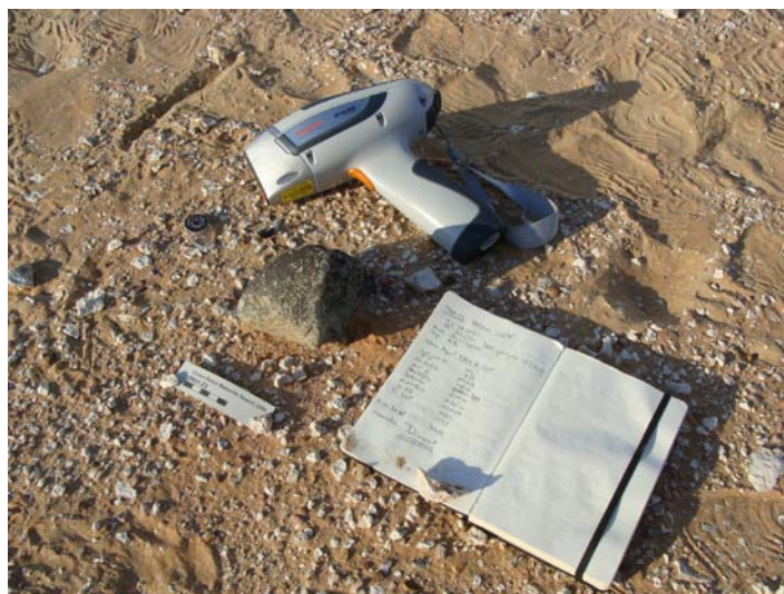
The diogenite RaS 287 with the HHXRF and the field book where its classification is noted.
