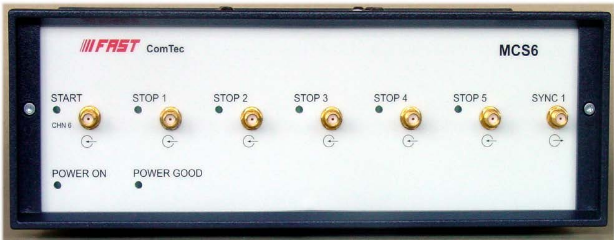
Figure 5.5: Front panel view of the FastComTec ® TDC with multi stop inputs. External trigger signal from pulse generator has to be connected to the START connection and spectrometer signal from the anode has to be connected to one of the STOP inputs.
