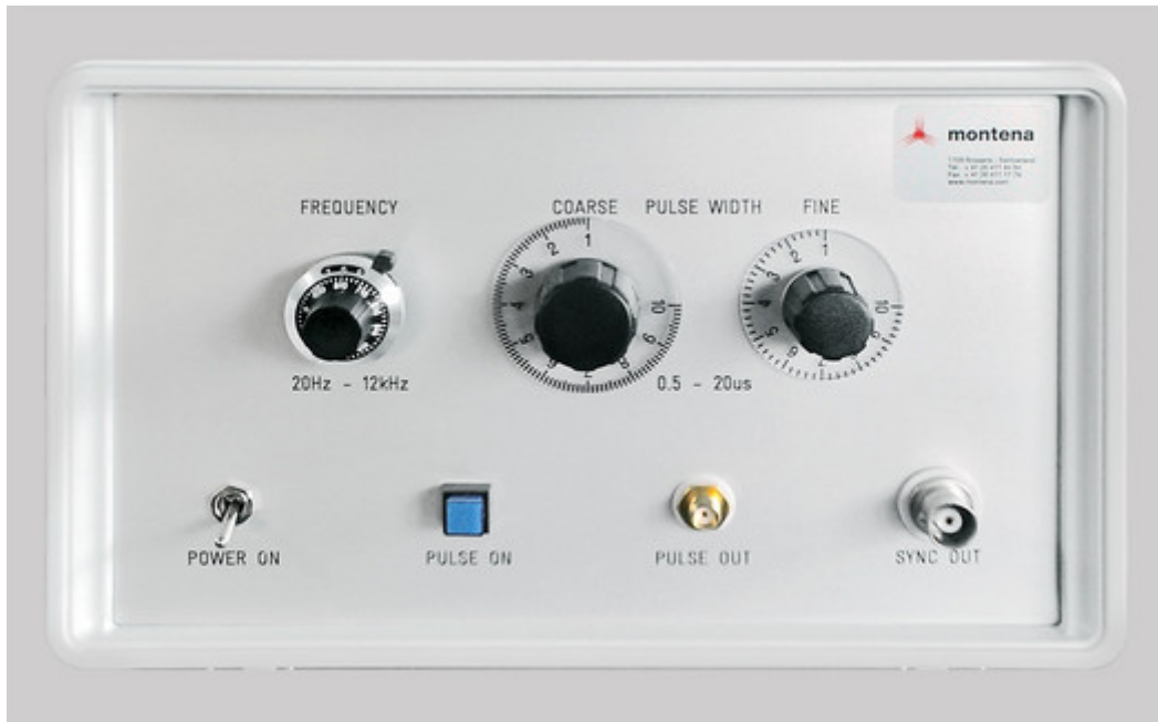
Figure 5.6: Front panel of the pulse generator from Montena ® . PULSE OUT and SYNC OUT are for pulse and trigger signals. The back panel has three connections, one for ground, one for the bias voltage, and one for the high voltage power supply.
