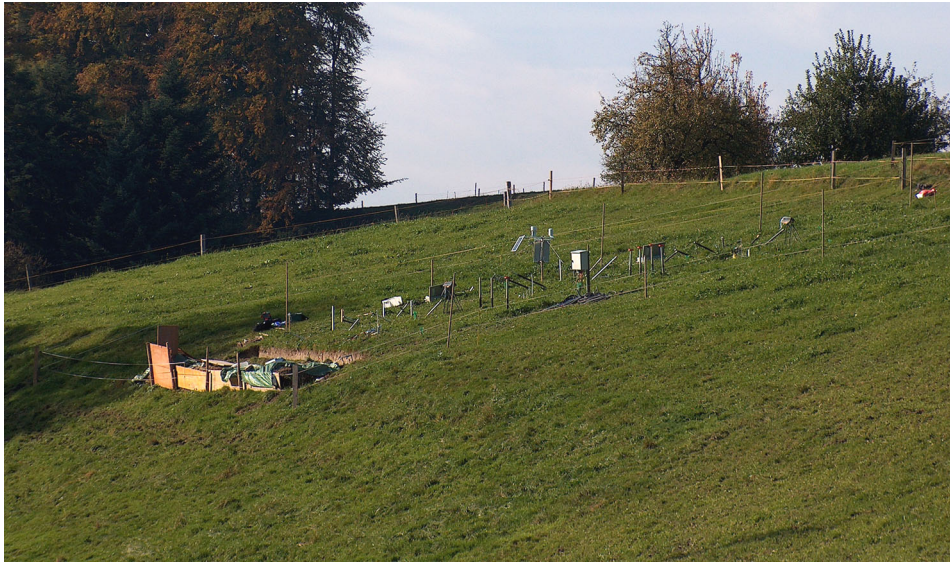
Figure 2.1. The Lutertal study site on a grassland slope in northern Switzerland. Note the brownish trench face which was excavated at the bottom end of the instrumented 100 \text{ m}^2 plot.
